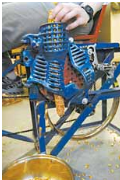
TINKERERS: Howard Kellog (right) and lab partner Lisa Tacoronte devise the mechanics for a bike-powered corn sheller (left) in MIT's D-Lab.
